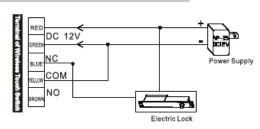
Wireless touch switch connect with electric lock
