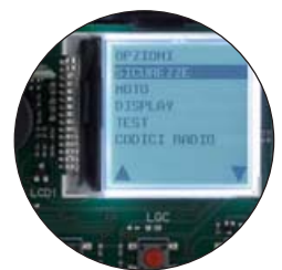
SELF-PROGRAMMING MONITORED BY AN LCD GRAPHICS DISPLAY ELDOMSDG/6
