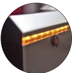
HOOD WITH BUILT-IN BOOM MOVEMENT LEDS
