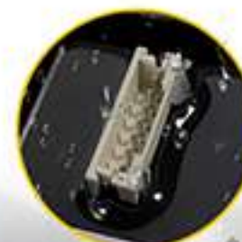
Rear cover resin sealant
